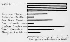
Fig. 48.—Relative cost of producing a given amount of light by various illuminants at usual prices. Costs are based on the following prices: Candles, 12 cents a pound; kerosene, 15 cents a gallon; gas, 81 for 1000 cubic feet; electricity 10 cents a kilowatt hour. The solid lines represent cost of fuel or of current, the shaded parts the cost of the mantles and bulbs. Where prices are different from those given above, costs will be correspondingly different.
