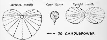
Fig. 46.\*—Comparison of amount of light given by different gas lamps. Each lamp is supposed to burn 5 cubic feet an hour, costing ½ cent if gas is \$1.00 a 1000 cubic feet. Note that the mantle lamp gives four or five times as much light as the open flame. The inverted mantle gives more light downward and less upward than the upright mantle.
