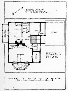
Fig. 7.—Second floor plan, showing sleeping area.
