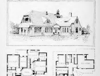
Fig. 8.—A farmhouse plan, showing diagonal corners used deliberately for purpose of design.
