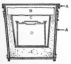
Fig. 49.—Diagram of a home-made fireless cooker. A, outer case; B, cushion; C, cooking compartment; D, food container; E, packing material.
