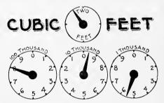
Fig. 42.—Gas meter index reading 79,500 cubic feet.
