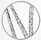
Fig. 59.—Wool fiber, showing the characteristic scales and the serrated surface.
