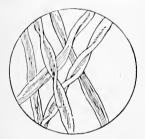
Fig. 57.—Cotton fibers, showing the characteristic twist.
