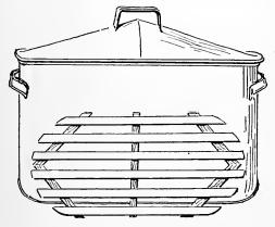
Fig. 123.—Sterilizer, showing false bottom as a rack.
