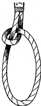
Half Hitch and Seizing —A simple, semi-permanent loop.
