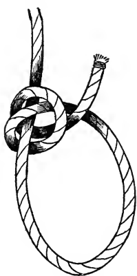
Midshipman's Hitch —A much better way of making the above, for the rope jams itself, and there is but little strain on the seizing. A man overboard catching a rope can make this—passing the bight between his legs and pressing the ropes together in his grasp in place of seizing. He could not tie a bowling or a noose unless he had slack.
