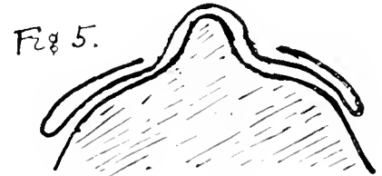
Fig 5. SECTION OF BACK SHOWING METHOD OF FOLDING BLANKET TO RAISE ARCH OF SADDLE TEMPORARILY ABOVE THE WITHERS.
