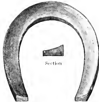
Fig. 634.—A Bad Foot Surface
