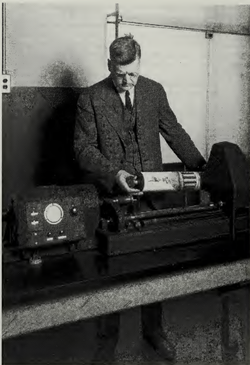
Figure 1 — Sending apparatus for 70B-1 telephotography equipment. Preparations are being made by J. H. Bell to send the picture of "Golden Boy". May 2, 1934. Photo courtesy of AT&T Archives.
