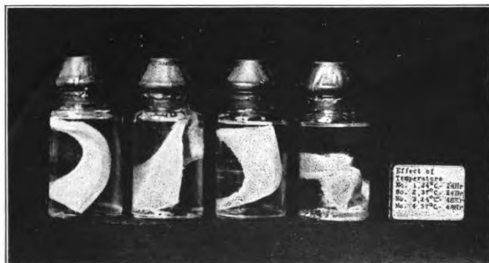
Fig 4.—Left-hand bottle stood 24 hrs at 24° C. in H 2 O and 24 hrs. in lime. Next bottle stood 24 hrs. at 37° C. in H 2 O and 24 hrs. in lime. Next bottle stood 48 hrs. at 24° C. in H 2 O and 24 hrs. in lime. Right-hand bottle stood 48 hrs. at 37° C. in H 2 O and 24 hrs. in lime.
