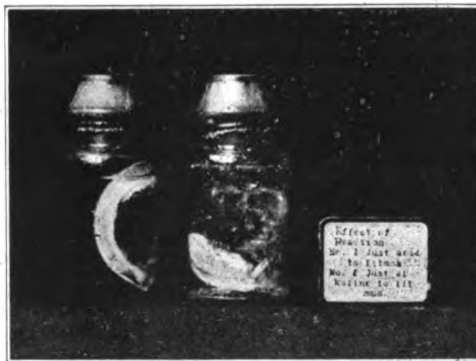
Fig. 5.—Solution in left-hand bottle just acid to litmus. Solution in right-hand bottle just alkaline to litmus.
