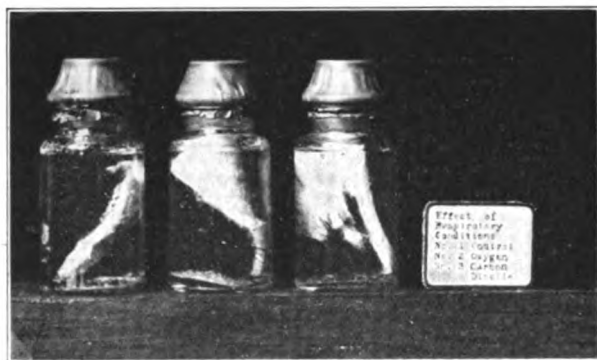
Fig. 7.—Hide shown at left stood in water. Hide shown in middle stood in water + continuous stream of O_2 . Hide shown at right stood in water + continuous stream of CO_2 .
