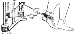
Illustrating Method of Fastening Foot and Leg Attachment to No. 5 Chest Weight Machine.
