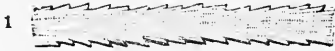
1. A fibre of long Merino, viewed as a transparent object by the microscope.
