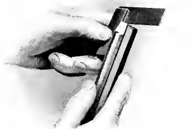
Grind the nose square to bottom and face
