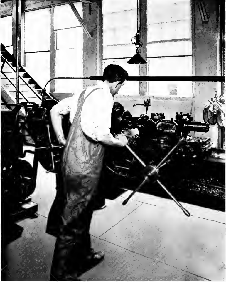
The Flat Turret Lathe at work, showing the convenience of control and the stability of tool support
