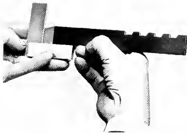
Grind the nose square to bottom and face
