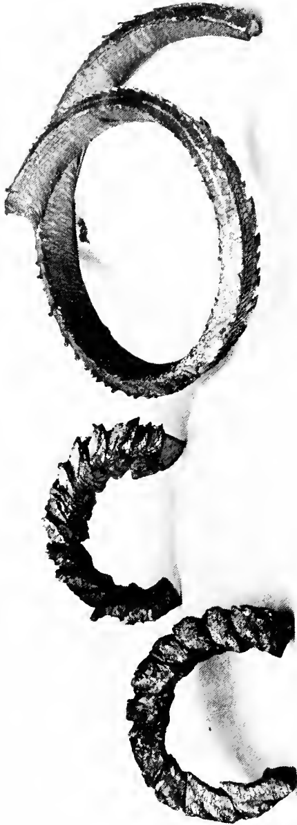
Characteristic Chips (about double size). Chips at the left made by diamond point tool having 70 degrees cutting angle. Chips at the right made by no-clearance tool, 45 degrees cutting angle
