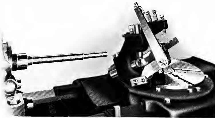
Turner adjusted to small diameter of work
