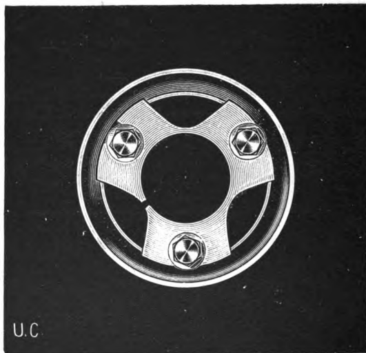
FIG. 423.—Sellers' compression coupling.
