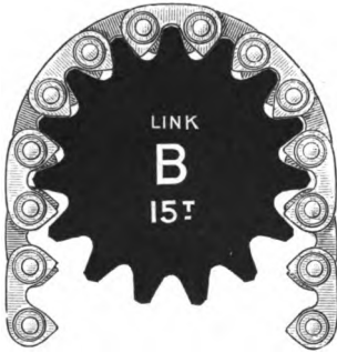
FIG. 457.—“Renold” patent silent chain.
