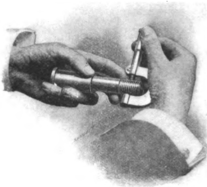
FIG. 96.—Micrometer gauging a screw.
