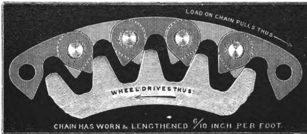
FIG. 461.—Worn and lengthened chain.
