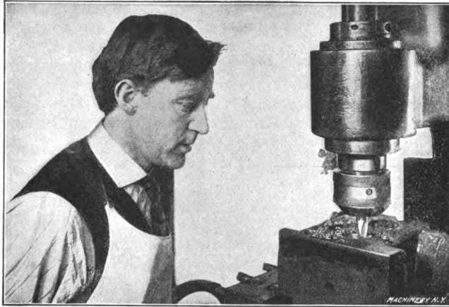
Fig. 12. Roughing out the Impression
