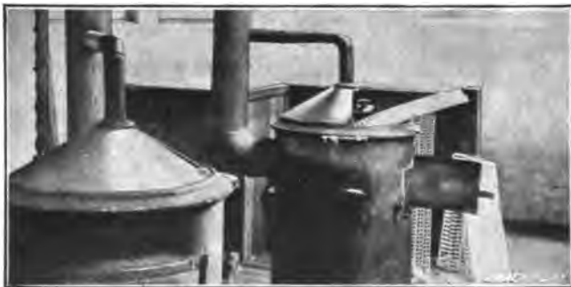
Fig. 41. Furnaces where the Tin Ingots are cast into Nine-pound Slabs
