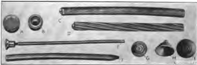
Fig. 38. A, B, C, and D, Steps in Making an Instrument Case by Extrusion; E and F, Extruded Parts for Automatic Pencils; G, Bullet Jacket; H and I, Hat-pin Guards
