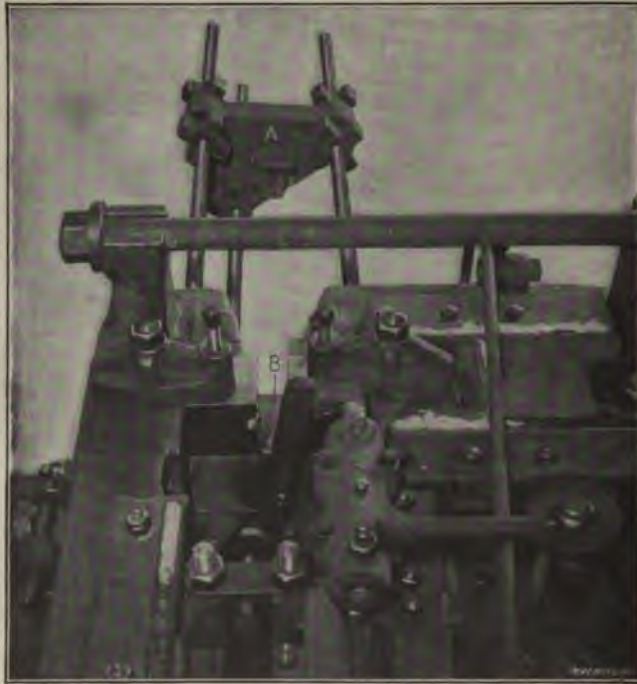
Fig. 10. View looking down into the Die Space of an Ajax Bolt Forging Machine
