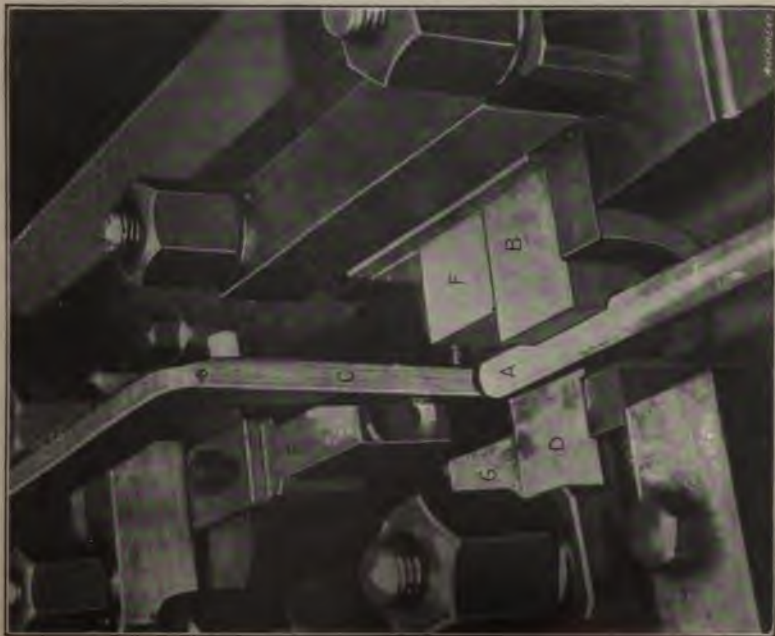
Fig. 6. First Step in the Production of Bolt Heads in Plain Forging Dies of the Type shown in Fig. 3
