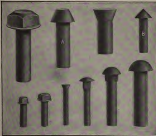
Fig. 33. Some Examples of Work which come within the Range of the Continuous-motion Type of Bolt and Rivet Headers
