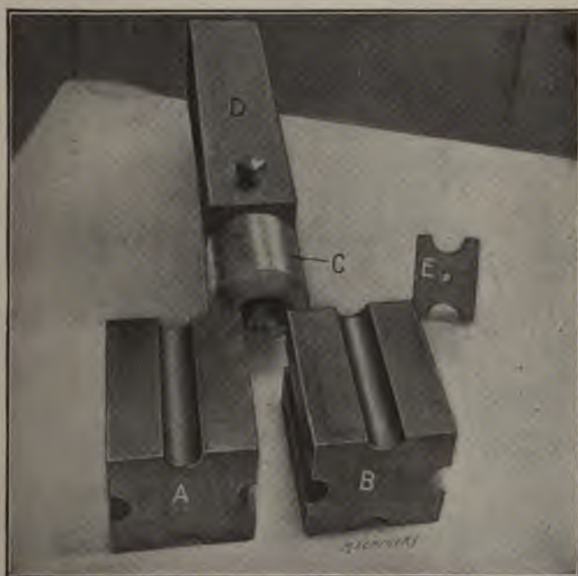
Fig. 25. Type of Dies and Tools used in the Continuous-motion Bolt and Rivet Header shown in Fig. 24
