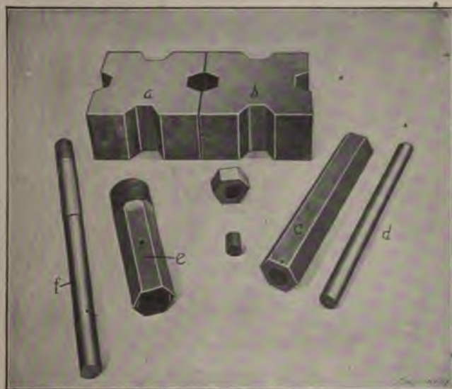
Fig. 42. Type of Dies and Tools used in making Hexagon Nuts in Center-fed Hot-pressed Nut Machine shown in Fig. 32
