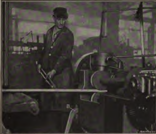
Fig. 30. Ajax Continuous-motion Bolt and Rivet Machine in Action making 1\frac{1}{2} -inch Rivets
