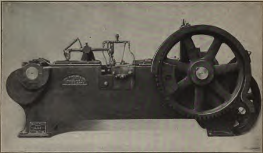
Fig. 34. Side View of "Ajax" Hot-pressed Center-fed Nut Machine showing Operating Side and Water Pipes for cooling Dies and Tools
