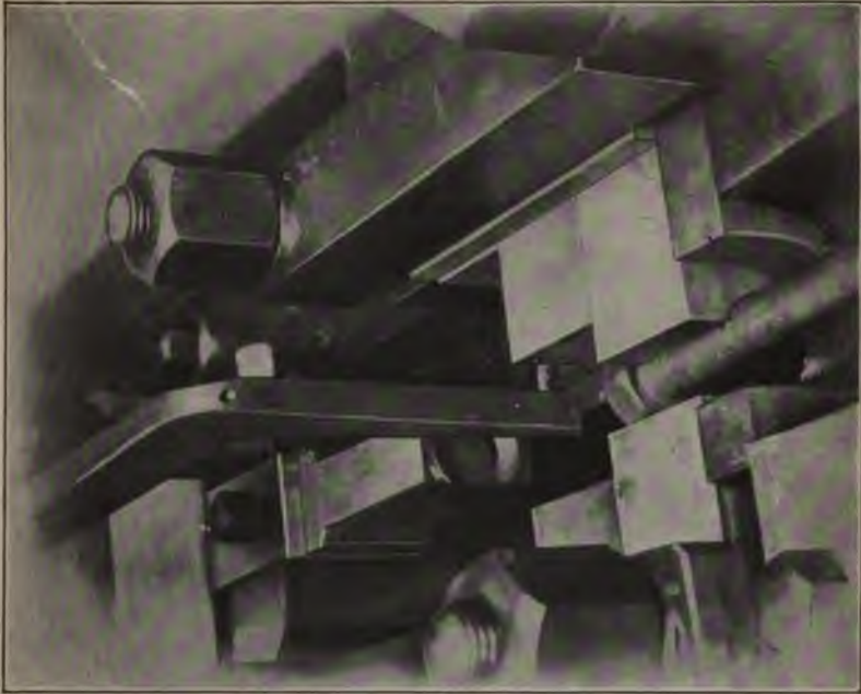
Fig. 7. Second Step in the Production of Bolt Heads
