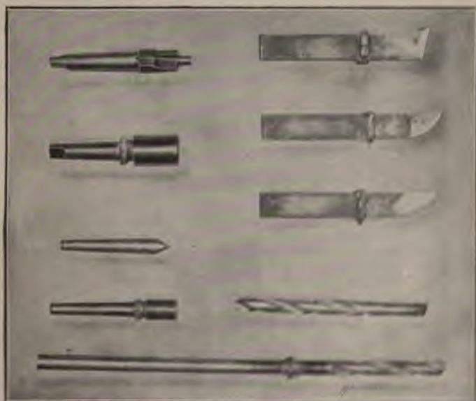
Fig. 5. Samples of Tools Electrically Welded for Economy of High-speed Steel and to effect Repairs
