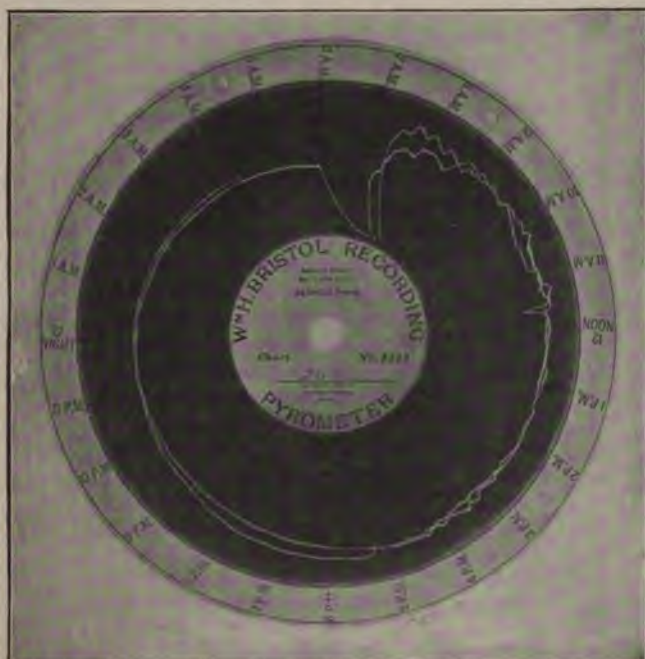
Fig. 3. Temperature Record obtained from an Annealing Furnace
