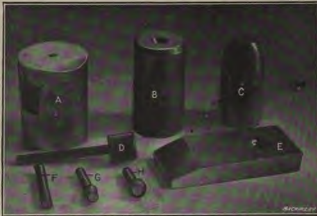
Fig. 33. A Set of Heading Tools and Work from a Double-blow Cold-header
