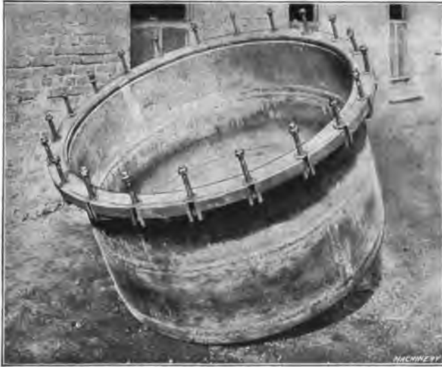
Fig. 17. Example of Welding Copper. Kettle is 5 feet 6 inches in Diameter, 31 inches deep and used under Pressure. All seams are welded on Both Sides
