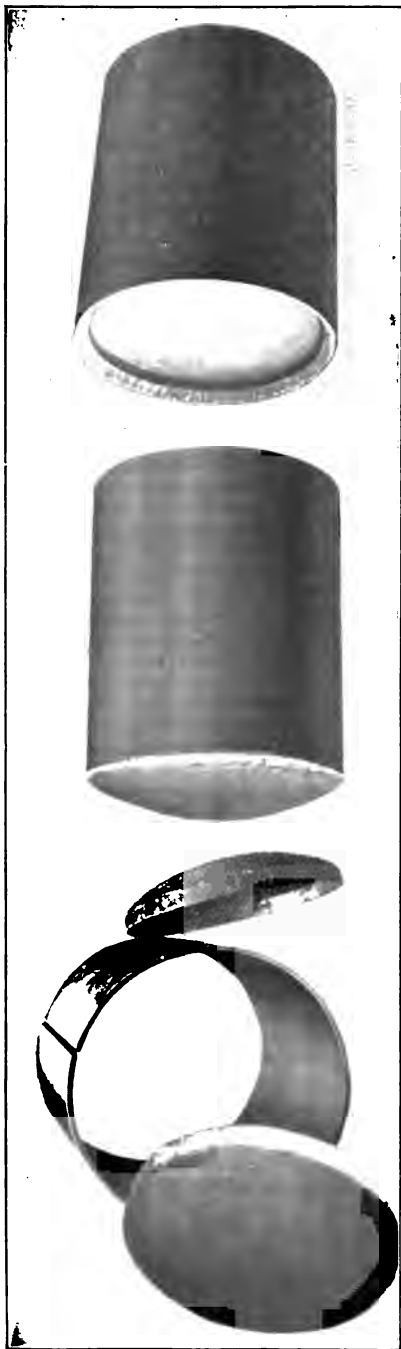
Figs. 11, 12 and 13. Progressive Steps in Making the Tank shown in Fig. 10
