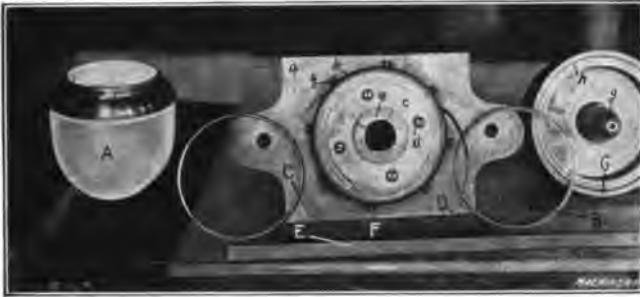
Fig. 30. Curling Die and Punch for a Steel Ring; Ring in its Various Stages of Formation; and Complete Wire Gas Globe in which Ring is used
