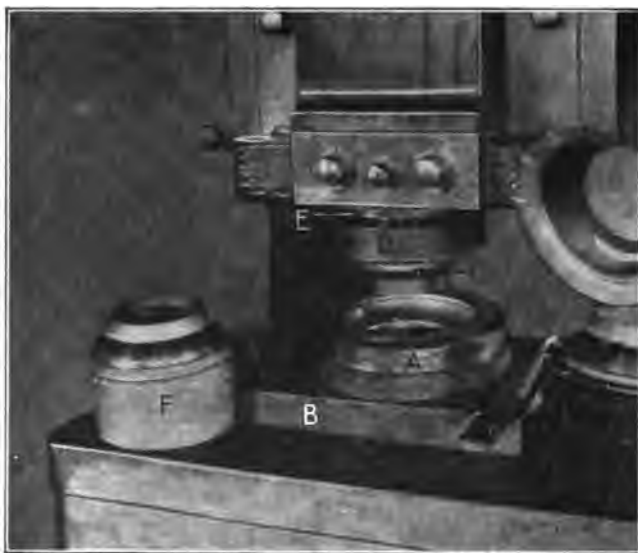
Fig. 32. Trimming Punch and Die for Brass Top set up on a Single-action Press
