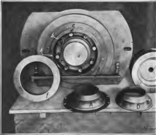
Fig. 29. Drawing Die and Punch and Brass Top after Drawing and Trimming Operations
