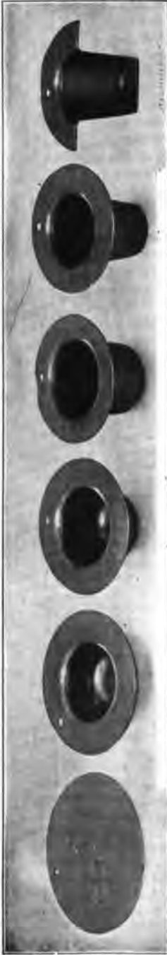
Fig. 6. The Successive Operations in the Production of a Flanged and Tapered Cylindrical Shell
