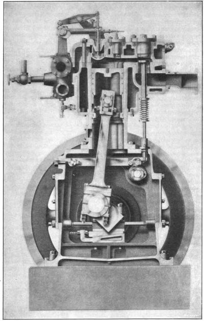
Fig. 2. Section through a Westinghouse Vertical Gas Engine
