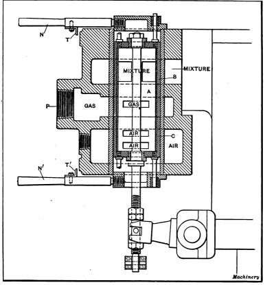
Fig. 6. Mixing Valve used on Westinghouse Gas Engine
