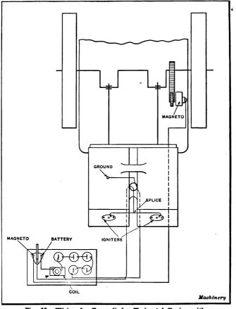
Fig. 13. Wiring for Two-cylinder Horizontal Engine with Batteries and Gear-driven Magneto
