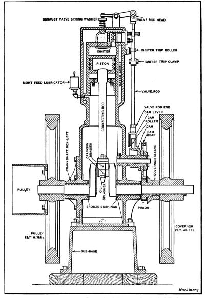
Fig. 3. Section through an International Harvester Co. Vertical Engine
