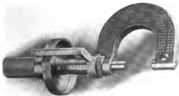
Fig. 24. Micrometer with Attachment for Reading Ten-Thousandths of an Inch.
