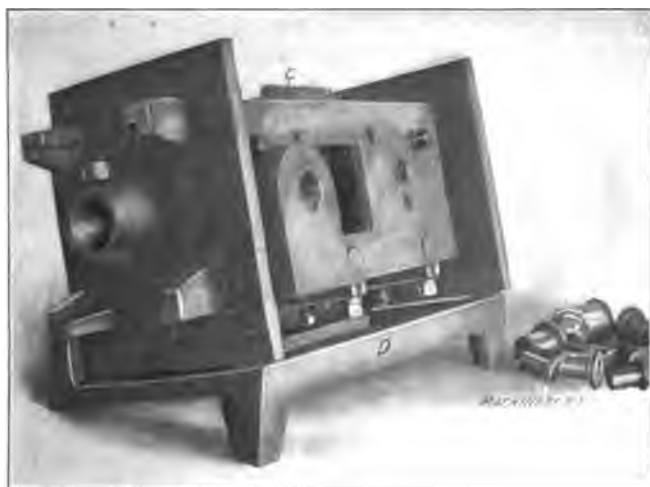
Fig. 108. Jig in Fig. 107 in Position for Drilling Holes at an Oblique Angle with Jig Base
