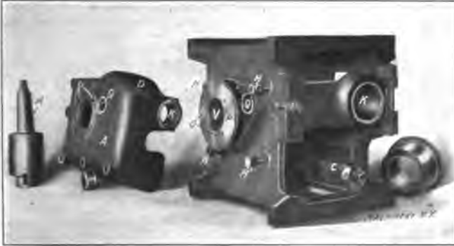
Fig. 103. Jig of Typical Design, and Work for which it is Used
