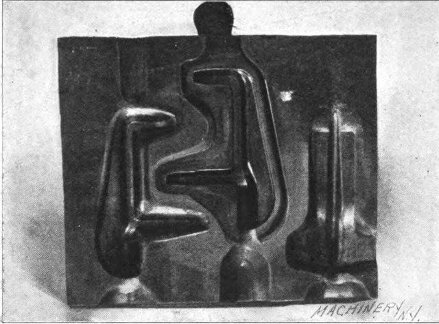
Fig. 52. Drop Forging Die Showing both Edging and Flattening Breaking-down Dies
