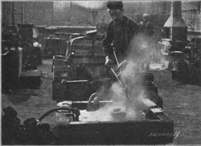
Fig. 60. Hardening the Face of a Drop Forging Die
