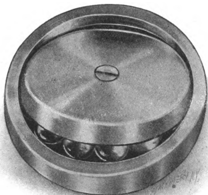
Fig. 43. View Showing Method of Assembling the R. B. F. Bearing. After the Outer Race is heated with Oil, the Balls and the Inner Race are Forced into Place, after which the Assembling Cup is removed
