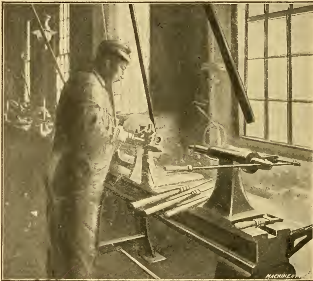
Fig. 34. Another View showing the Position of the Spinner and the Way the Tool is held when forming the Metal
