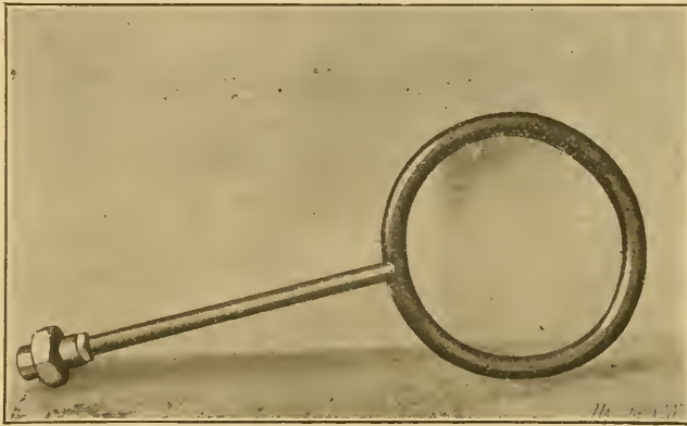
Fig. 17. Gas Burner for Heating Spinning Chuck
