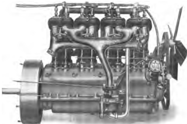
Fig. 14. Right Side of the Engine, showing Carburetor, Commutator, etc.
