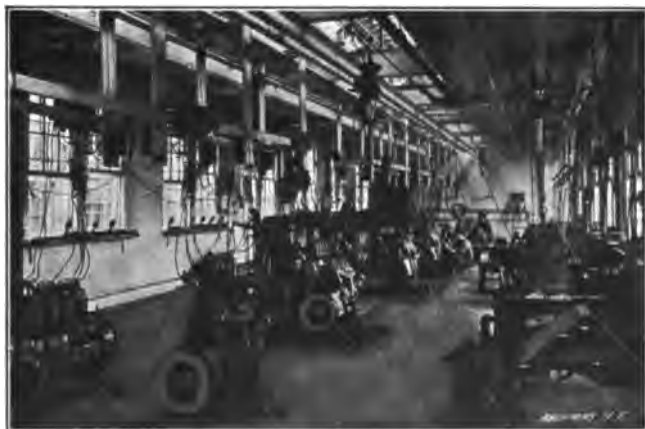
Fig. 5. Testing the Four-cylinder Engines
