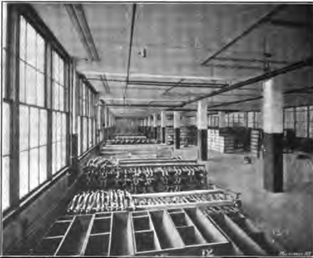
Fig. 36. View of Stock Room, showing Trucks in which Parts are taken to the Assembling Room
