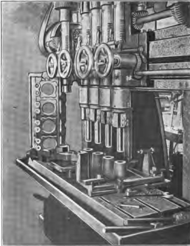
Fig. 21. Machine for Boring Frames
