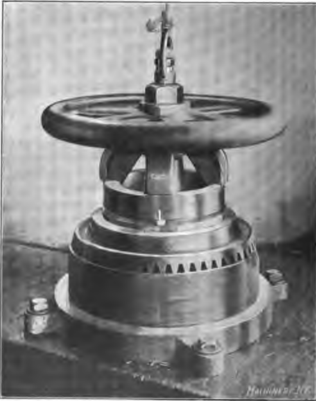
Fig. 44. A Convenient Fixture for Assembling the Gears on the Gear Case
