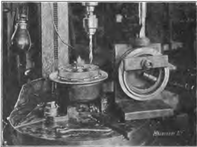
Fig. 34. Drilling the Three Oil Supply Holes in the Case (see Fixture at the Right), and Drilling the Bolt and Pivot Holes in the Cover
