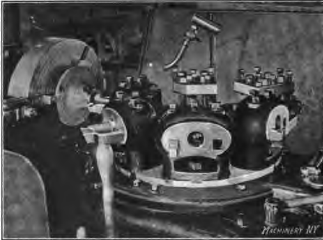
Fig. 35. The First Turret Lathe Operation in Finishing the Gear Case Covers
