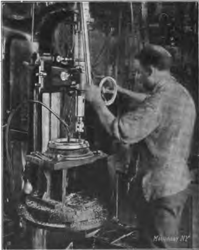
Fig. 45. A Tapping Operation and Operator with a Remarkable Record—75,000 Blind 5-16-inch Holes in Chrome-nickel Steel without breaking a Tap
