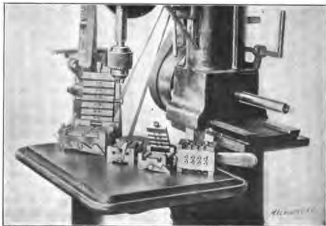
Fig. 26. Interesting Drill Jigs for a Simple Operation
