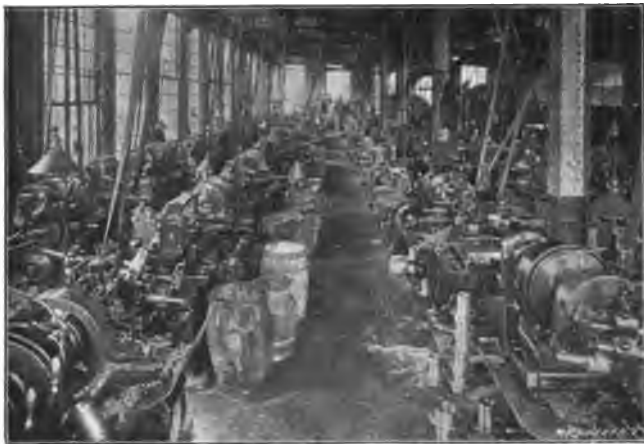
Fig. 28. An Unusual Array of Automatic Chucking Machines: Thirty-one are used in this Department
