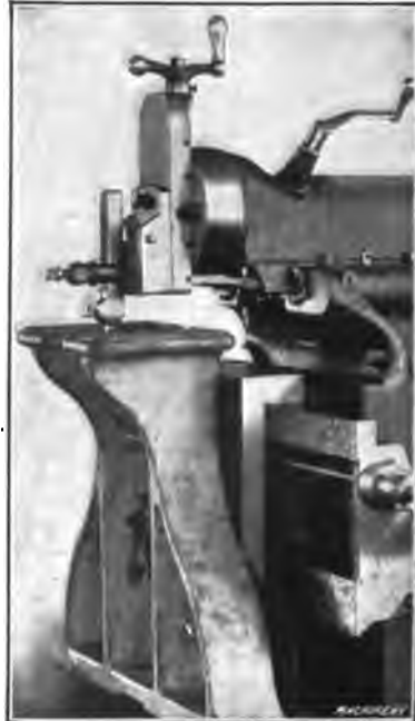
Fig. 46. Table removed and Casting Clamped to Cross-slide
