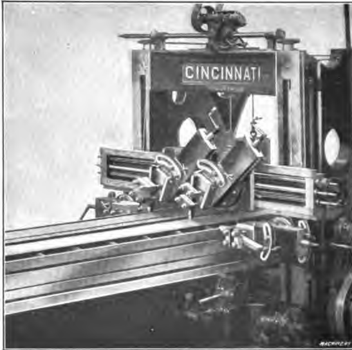
Fig. 12. Double-head Planer set for Planing Angular Surfaces
