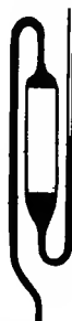
FIG. 19.—INCORRECT FORM FOR RESERVOIR OF BECKMANN THERMOMETER, THE UPPER PORTION OF THE RESERVOIR BEING TOO FLAT.
