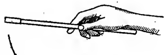
FIG. 21.—SHAKING A DROP OF MERCURY TO THE TOP OF RESERVOIR. (From Biltz.)
