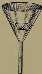
Perforated disk in ordinary funnel.
