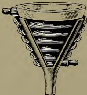
Jacketed funnel for hot water or steam.
