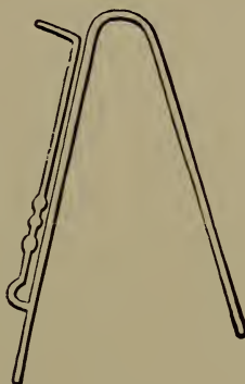
Glass siphon with lateral suction tube.
