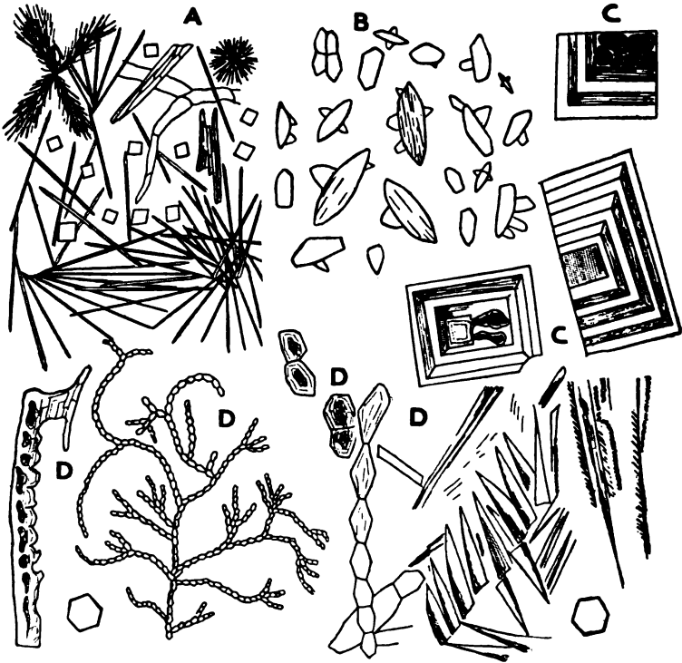
FIG. 327. Crystals of some of the common reagents which not infrequently separate on the slide and may be mistaken for cell contents: A, isotropic crystals of chloral which occur in cubes about 10\ \mu in diameter or long needles about 50\ \mu long; B, phlorogluccin which occurs in broad rectangular plates or ellipsoidal discs from 10 to 35\ \mu in diameter which are doubly refracting with a play of colors; C, cubes of potassium iodide which are isotropic; D, crystals from potassium hydrate solution which separate in broad prisms and branching chains that are doubly refracting and give marked color effects.
