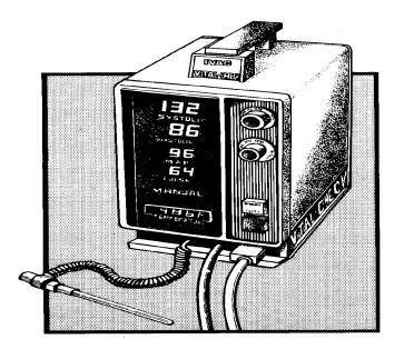
Figure 4-3. Electronic vital signs monitor.
