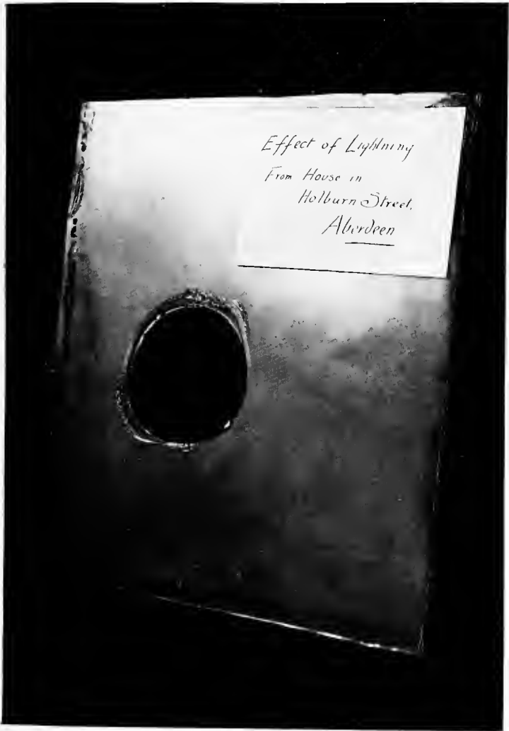
Fig. 93.—Effect of lightning on window pane
