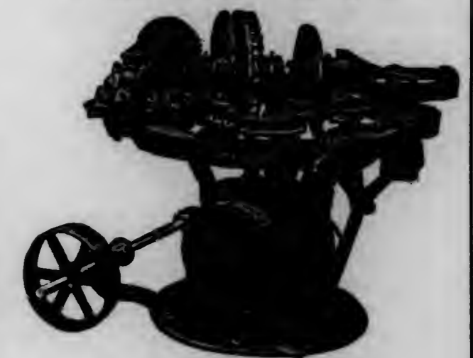
NEW "ORAM" RAPID BILGE-HOOP REMOVING MACHINE
