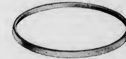
KEG CROZER—4-inch Diameter Head to 11-inch Diameter Head and Up to 20-inch Long Staves
