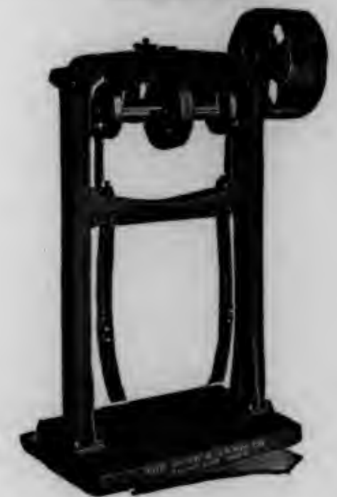
NEW "ORAM" RAPID BILGE-HOOP REMOVING MACHINE
