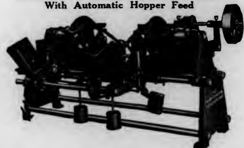
ROSIN BARREL STAVE CROZER With Automatic Hopper Feed
