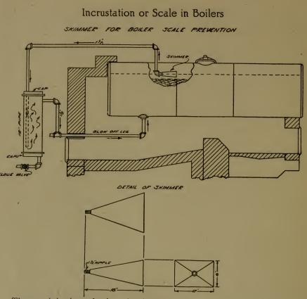
The precipitation of mineral substances or mud that is held in solution by boiler feed water is the cause of scale or incrustation.
