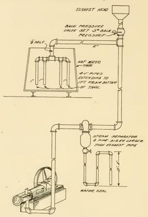
Beyond any reasonable doubt the Troy Hot Water System will solve the problem of hot water in the laundry plant and further, as the hottest water is always being circulated through the piping right at the washer, there is always hot water available at the valve when the operator opens the valve.
