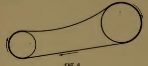
In figure "A", a belt is shown running in the proper direction and the belt is in the good condition which allows a good contact with the pulleys.
