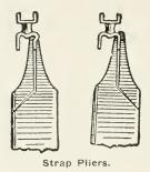
special pliers the bending and paralleling of the straps can be done all at the same time without likelihood of breaking the straps.
