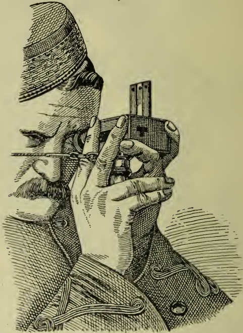
Showing the correct position of the hands in holding the Right Angle Instrument.
