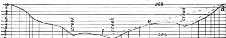
FIG. 192. SECTION from J. CRAWFORD to hill 388 east. Hgts to Dsts as 15 to 1.
