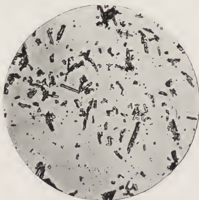
No. 67. CALCIUM SULPHATE — Photomicrograph \times 300 . Pptd. from cold, moderately concentrated solutions.
