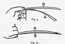
at the free end (see Fig. 9), but if the grain runs the long way in the under piece the free ends will not part (see Fig. 10). This is because paper is stiffer across the grain. The experiment is a good method of telling
