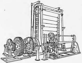
Fig. 8. Stack of calender rolls.
