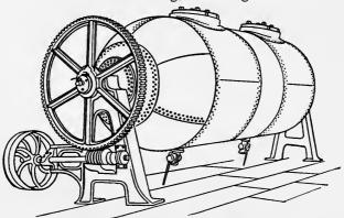
Fig. 2. Revolving Boiler for "cooking" rags.
