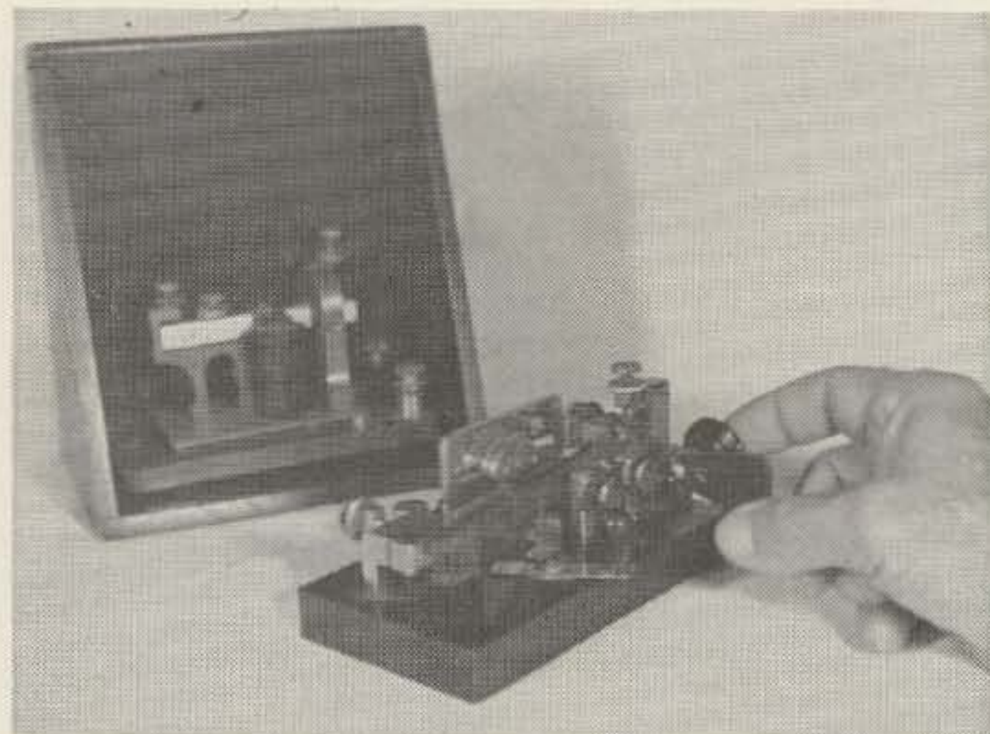
Early Mecograph Key—1906. Popularly called "The Right Angle Bug" by telegraphers. This is the first of three models made by the Mecograph Company.
