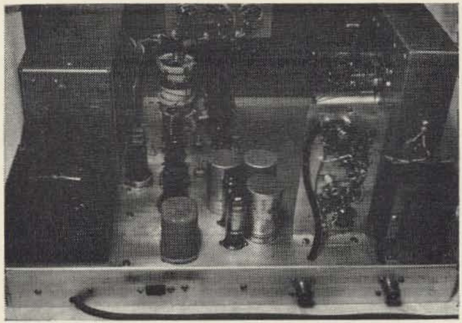
Fig. 2—Rear view: The stepping relay is in the case in front of the power transformer. All shields have been removed for this and all other photographs. The Nixie panel is visible on top of the front panel. Sockets on back are in order: switched 115VAC for linear, 50-239 output to 14 mc receiver, and 50-239 input from SSB exciter. 144 mc output is on subchassis.
