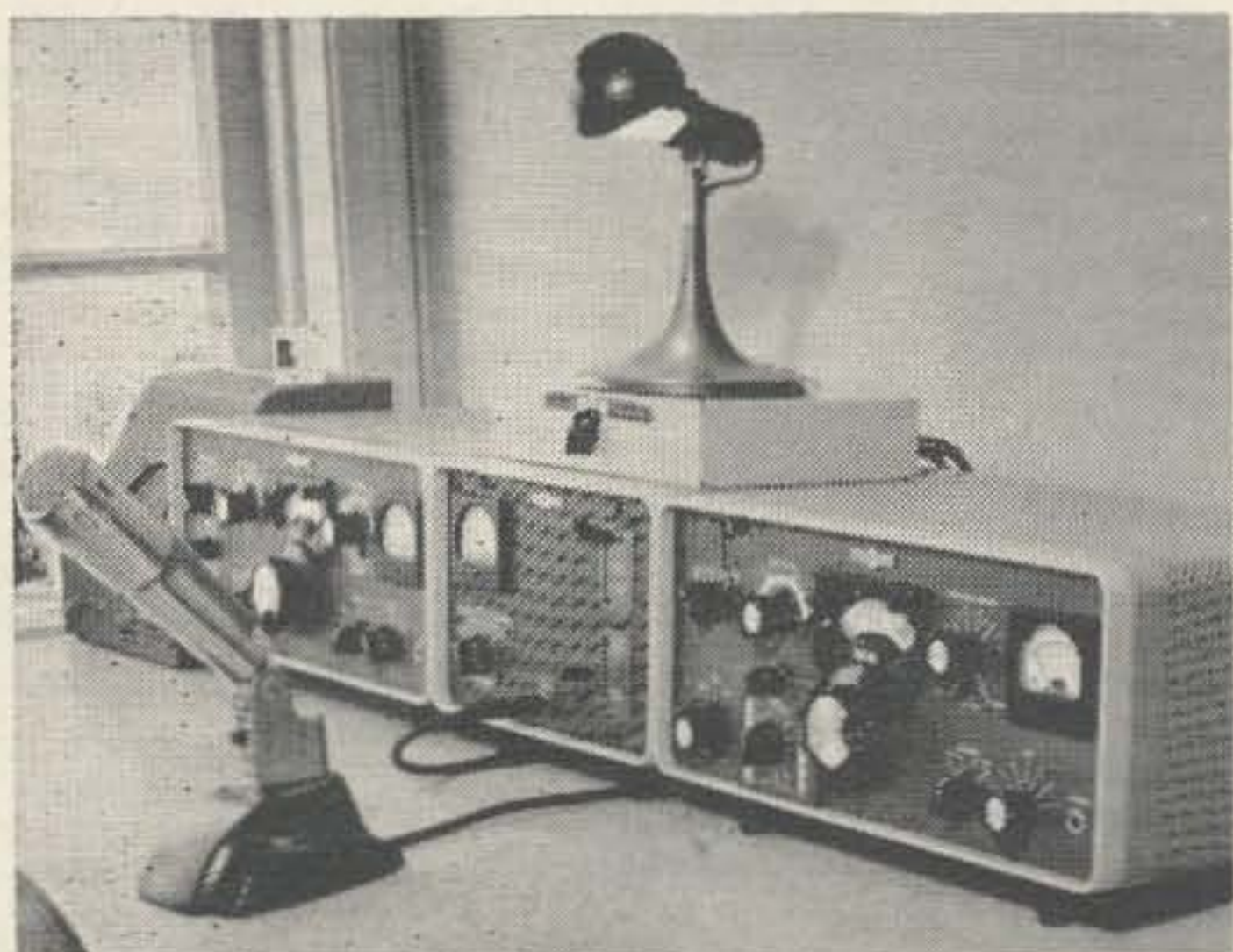
The switching box on top of the SWR bridge.
