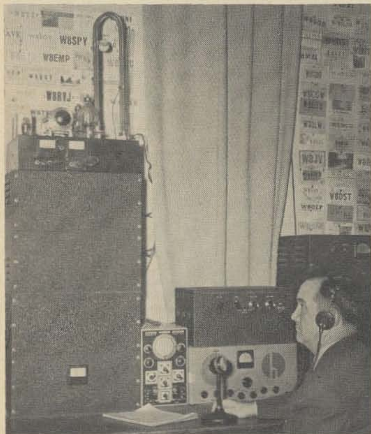
Actually, operation of the amateur station at the New York World's Fair began in 1938, long before the fair opened. At this time all transmissions from W2USA were sent out on five meters and picked up and relayed by other stations on all the other bands. Here Ed Dunn, W2ETD, is operating the 400 watt five-meter phone station donated by W2DKJ. Directly in front of Ed is the Hallicrafters 5-10 receiver and National speech amplifier. The five-meter antenna was an extended double Zep, designed by Frank Lester, W2AMJ, and fed with a long hunk of electric light wire. Note the great number of QSL cards from the 8th district which acknowledged the 5-meter transmissions—either direct or by relay.
