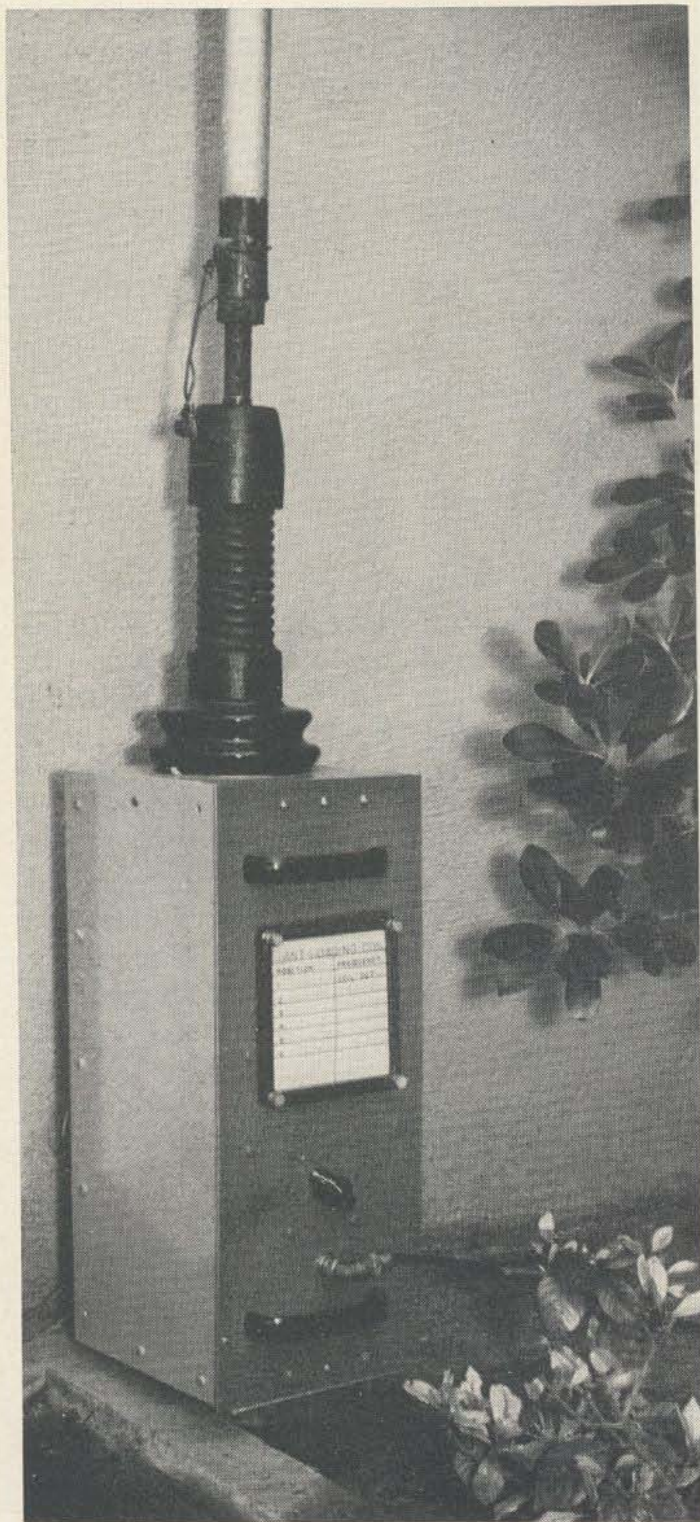
The base of the un-guyed vertical antenna.
