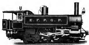
RACK LOCOMOTIVE WITH TWO COG-WHEELS
