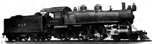
BALANCED COMFOUND ATLANTIC TYPE LOCOMOTIVE For the Atchison, Topeka and Santa Fe Railway
