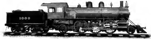
COMPOUND PRAIRIE TYPE LOCOMOTIVE For the Atchison, Topeka and Santa Fe Railway
