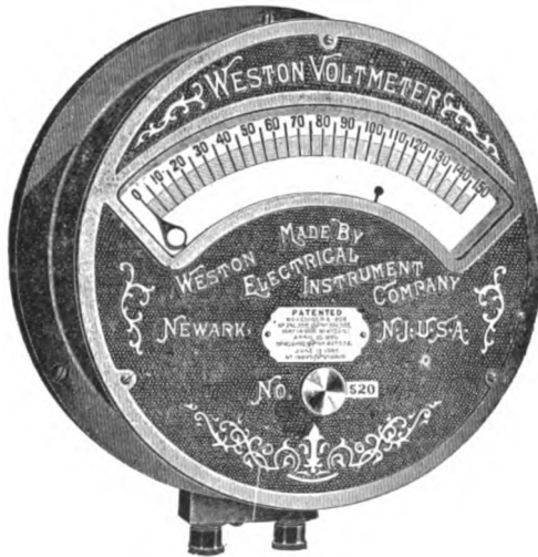
FIG. 336.—WESTON VOLTMETER. mediately without any swing. To find the difference
