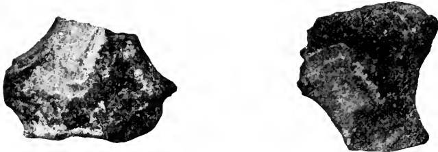
FIGS. 5 AND 6.—PIECES OF SCALE FROM THE FIRE SPACE OF A YARROW BOILER. (NEARLY FULL SIZE.)
