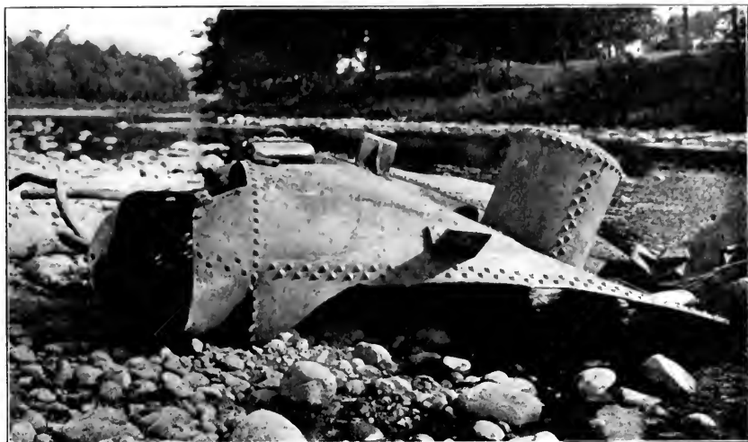
FIG. 3. THE EXPLODED BOILER, SHOWING RUPTURE.
