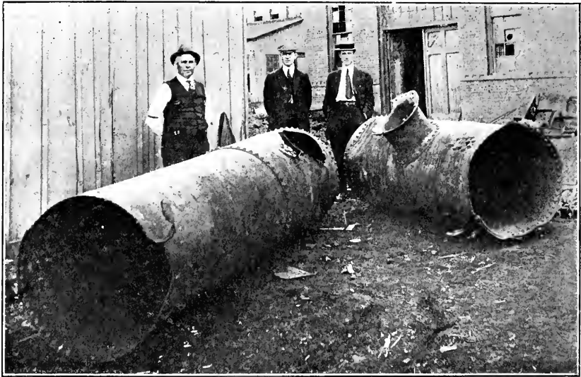
FIG. 2. PORTIONS OF EXPLODED STEAM DRUM, LONDONDERRY EXPLOSION.
