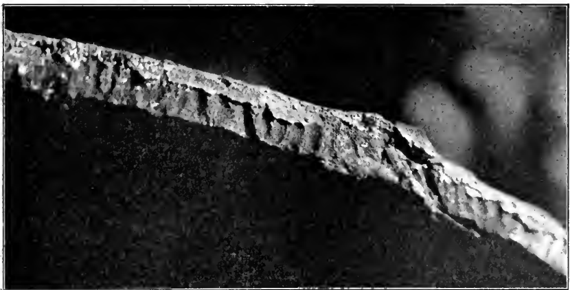
FIG. 2. EDGE VIEW OF RUPTURED HEAD.
