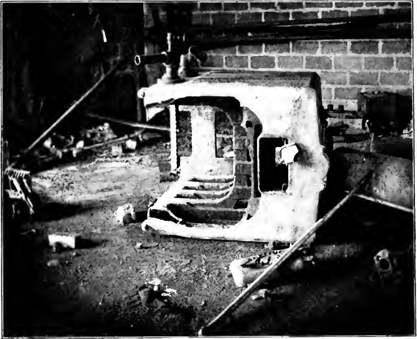
EXPLODED HEATING BOILER.
