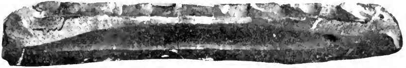
Figure 2—Closeup of the break in the part which went through the casing. A progressive fracture is clearly visible here, but it was so hidden before the accident that no inspection procedure short of taking out the blades could have led to its discovery.
