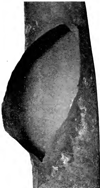
Tube failure which had serious consequences.
