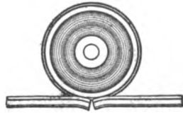
Tendency which the motion of the wheel has to crush the rails at their joint.
