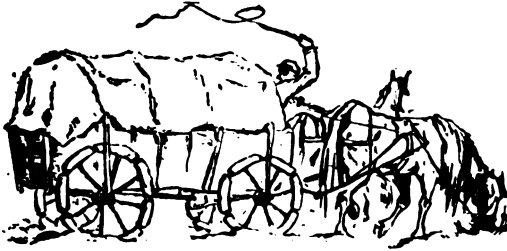
A Servian wagon. It is constructed wholly of wood except a rude metal spring. The octagon and oblong wheels to be met with in western China vie with the above in oddity.
