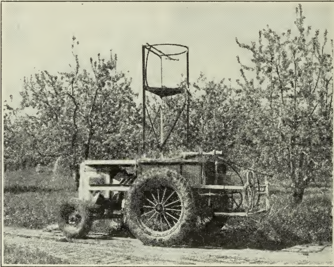
Fig. 13.—An auxiliary-engine-powered 35-gallon-per-minute sprayer mounted on pneumatic tires. The rear tires are tractor type. The tank capacity is 300 gallons. The tower is incorrectly mounted: it should be turned 180 degrees so the leg in the rear would be the leading leg. Even less damage to branches and fruit would result if the base of the tower was covered with sheet metal.
