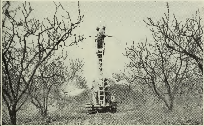
Fig. 14.—Large sprayer with tower permitting spraying as the rig moves continuously. The tower can readily be lowered by folding over on the top of the sprayer. (Courtesy of C. B. Weeks.)
